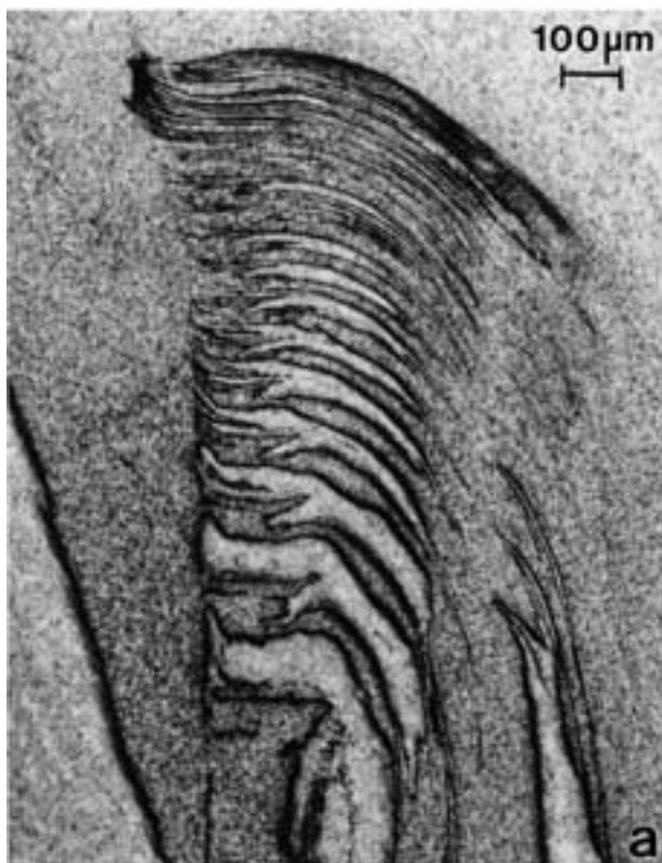
Figure 20 Examples of residual, complex flow features following FSW. (a) Cu blocks and shear features in the DRX brass zone of FSW of Cu and brass (70 Cu 30 Zn). (b) Complex flow patterns for FSW of 7050 Al and 7075 Al. (c) Complex flow zone in Cu/Al FSW. (d) Complex flow showing intercalation of Ag and brass shear structures in FSW of Ag/brass. (Continued.)
