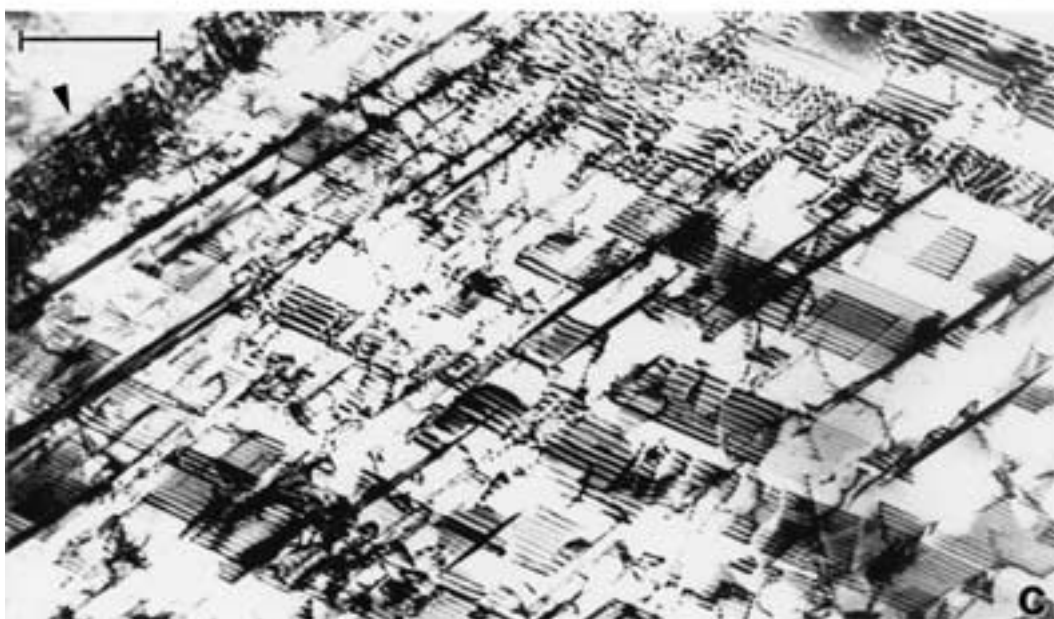
Figure 2 Continuation of thin foil (TEM) 304 stainless steel tensile specimens showing dislocation and related microstructure (ledge) variations at grain boundaries (arrows) corresponding to engineering strains noted. (a) \epsilon = 1.5\% , (b) \epsilon = 2\% , (c) \epsilon = 6\% . Magnifications are indicated in (a). All matrix crystallographies and diffraction conditions are the same and as noted in Fig. 1a.
