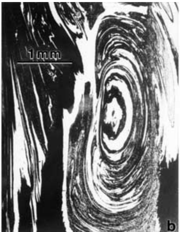
Figure 20 Examples of residual, complex flow features following FSW. (a) Cu blocks and shear features in the DRX brass zone of FSW of Cu and brass (70 Cu 30 Zn). (b) Complex flow patterns for FSW of 7050 Al and 7075 Al. (c) Complex flow zone in Cu/Al FSW. (d) Complex flow showing intercalation of Ag and brass shear structures in FSW of Ag/brass. (Continued.)
